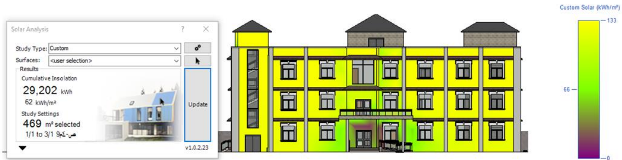
Figure 39: cumulative insolation for South Elevation in Winter.
