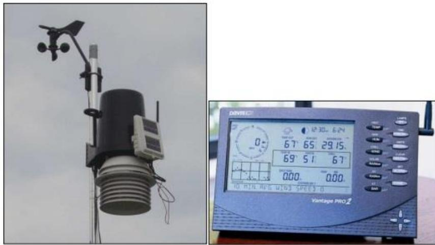
**Figure 2-2** Typical Wireless Automatic Weather Station Equipment ( Jenkins, 2015)
