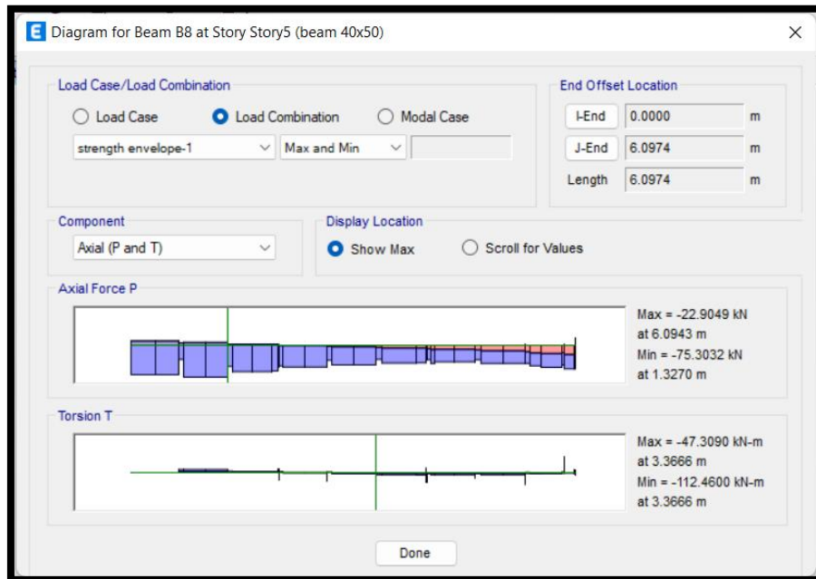
Figure 160: axial load on beam envelope strength combination
