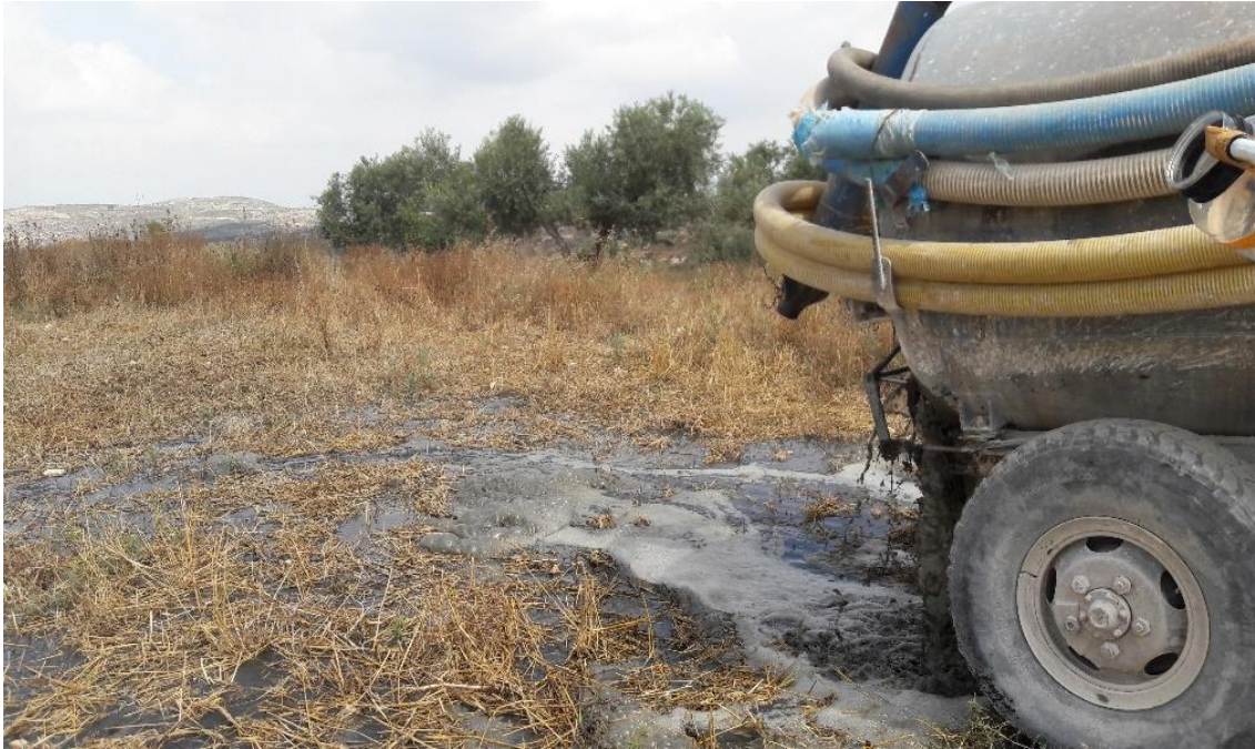
Picture 3.1: Disposal of septage on the land
