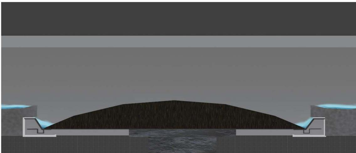
**Figure 5.9 Speed bump component to prevent water enter into system.**
