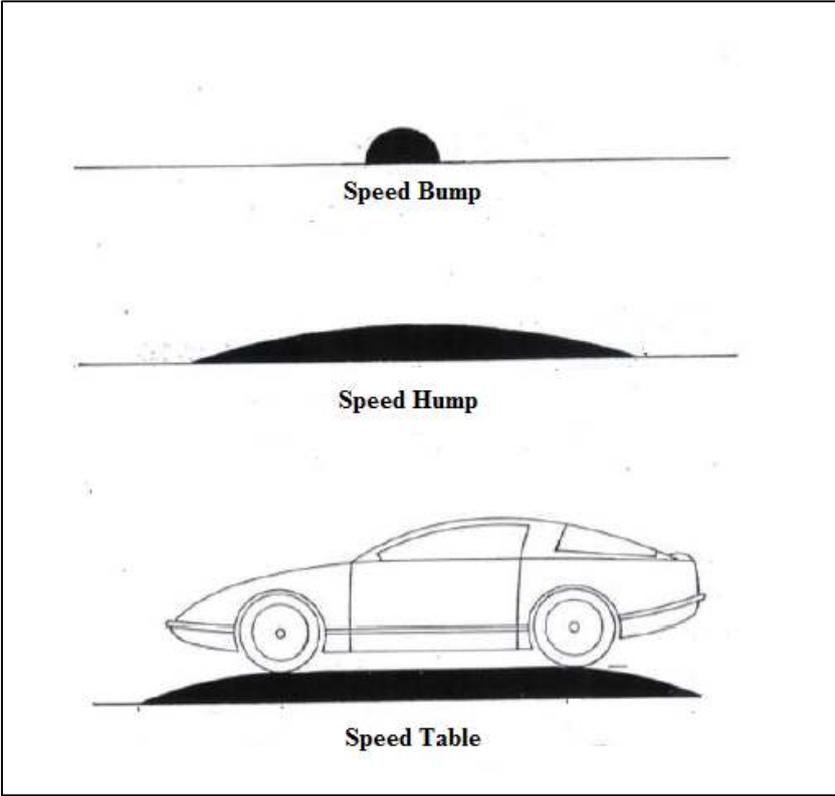
**Figure 1.1 Different common type of humps**
