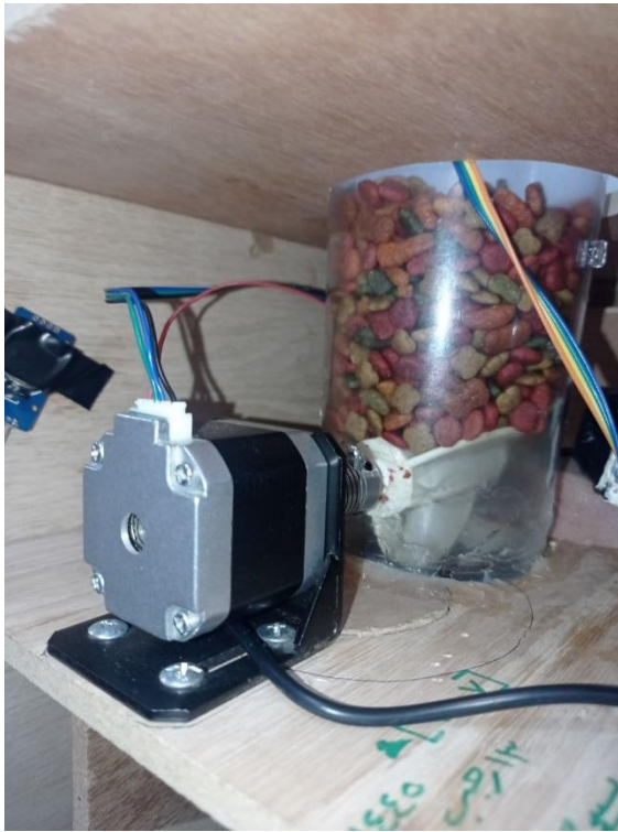
Figure 40 food dispensing mechanism
