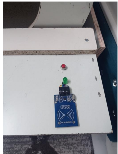
Figure 56 RFID with push button to turn on litter box
