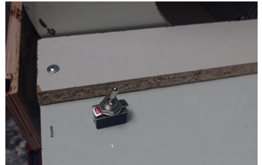
Figure 57 Switch button to control auto mode for the litter box
