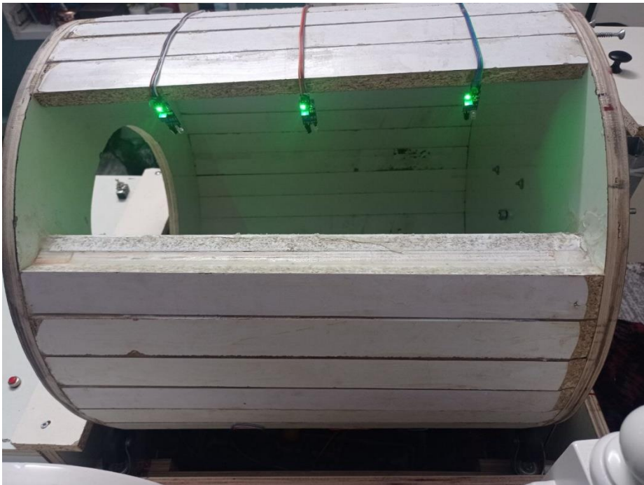
Figure 59 IR sensors to detect the cat's presence inside the device
