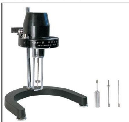
**Fig.(3.1):** NDJ - 1 Rotational Viscometer
