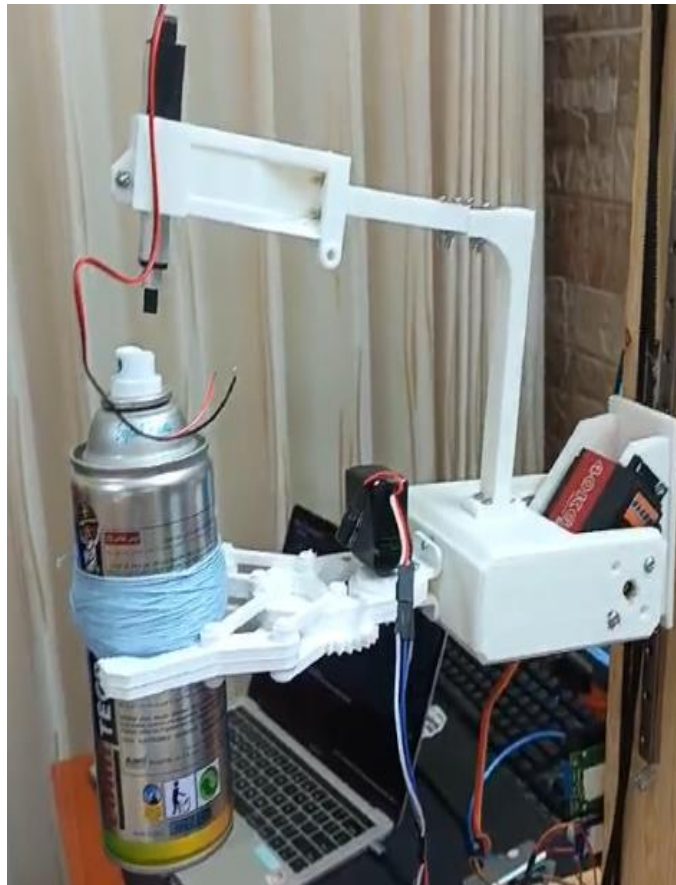
Figure 25: 3D-printed arm and gripper holding a spray can attached to the vertical axis.
