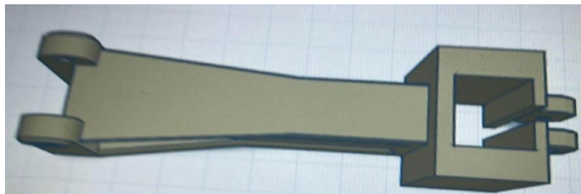
Figure 16: 3D-Printed Linear Actuator-to-Arm Linkage
