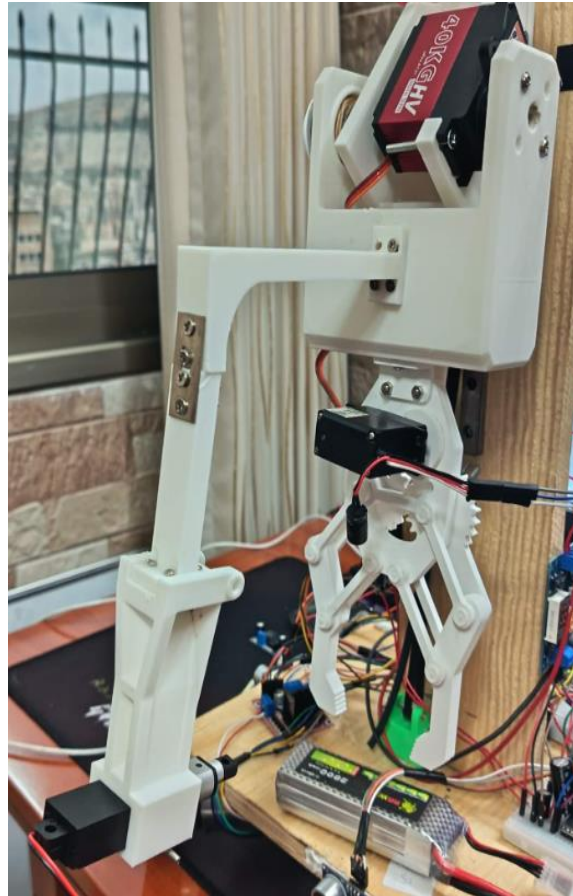
Figure 24: Close-up of the 3D-printed geared gripper mechanism with linear actuator.
