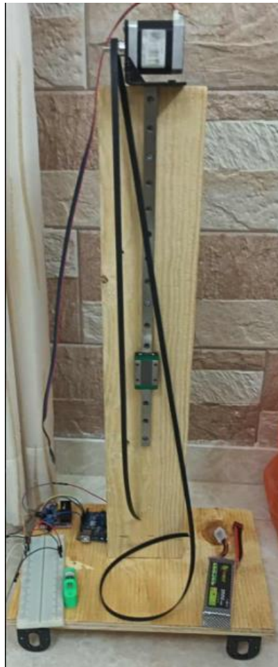
Figure 23: Assembled vertical linear axis with linear rail, NEMA17 stepper motor.
