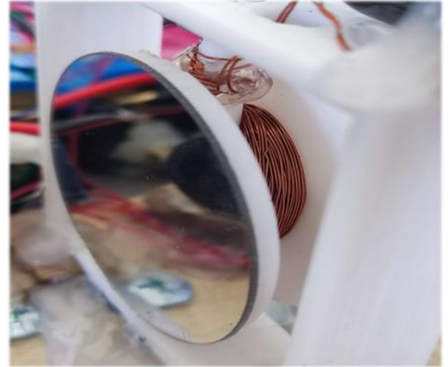
MEMS Mirror Desing Inspired By the DC Motor
