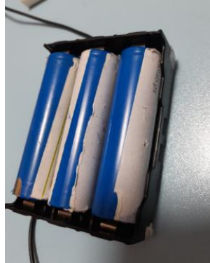
Figure 7: 3 battery everyone is 4volt to make 12 volt
