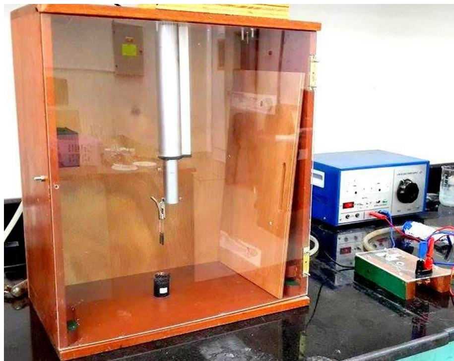
**Fig 3.2:** Local designed and manufactured dip coater designed at physics department by Mr. Mohammad Bahjat and Dr .Iyad Saadeddin.
