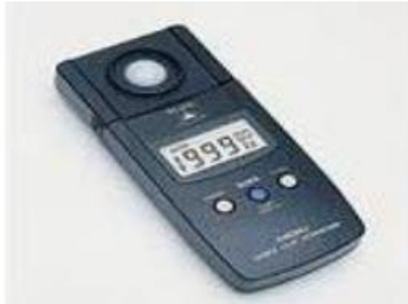
Fig. (3.2): Hioki 3423 Lux Hitester Digital Illumination Meter (Hioki 3423 Lux Hitester Instruction Manual, 2006)
