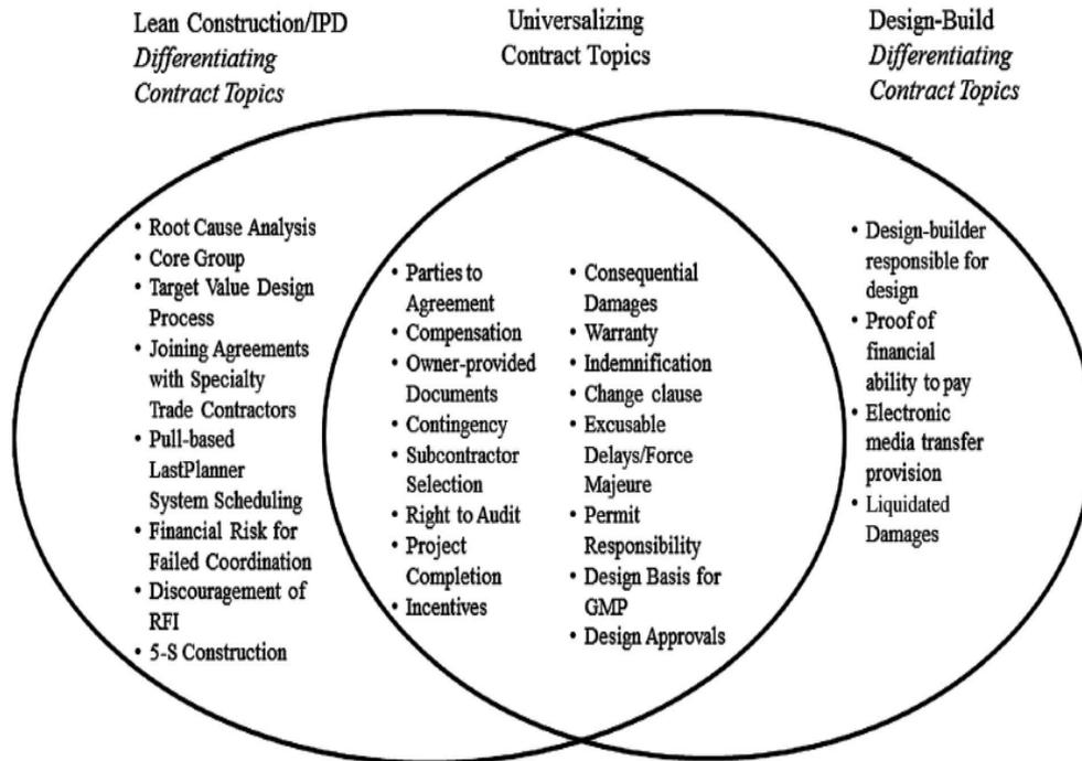
**Figure (2:8 ):** Comparative between lean construction contract and design build contract (Timothy et al ,2012)
