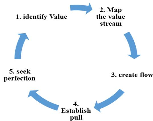
**Figure (3:2):** Lean construction Principles
