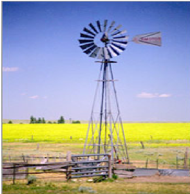
Figure(3.5): Multi-blade HAWT, for water pumping, Turpex company, South Africa
