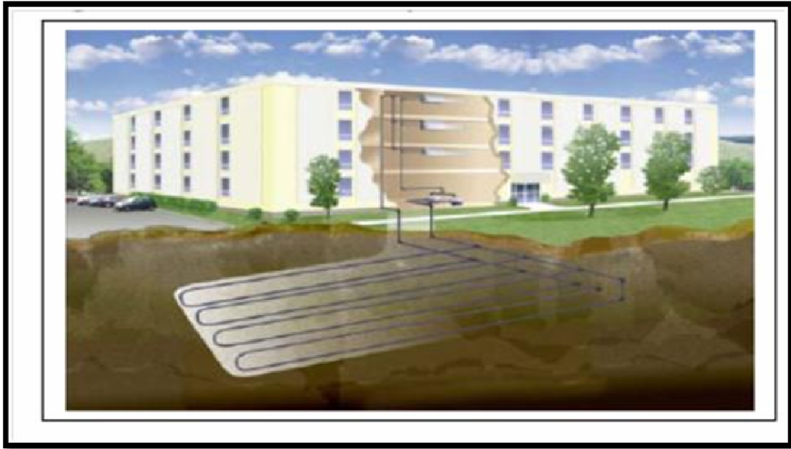
Figure (1.5) Horizontal Geothermal heat pumps [7]
