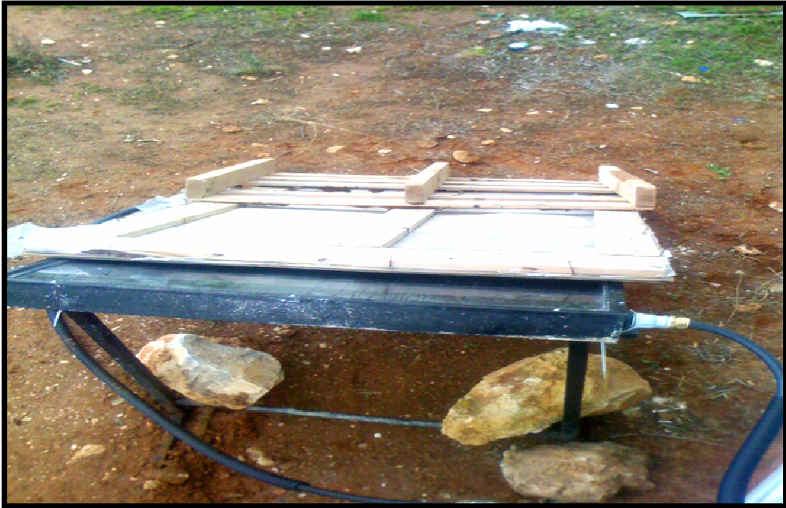
Figure (5.11) Local Solar water Heater 190x90 cm.
