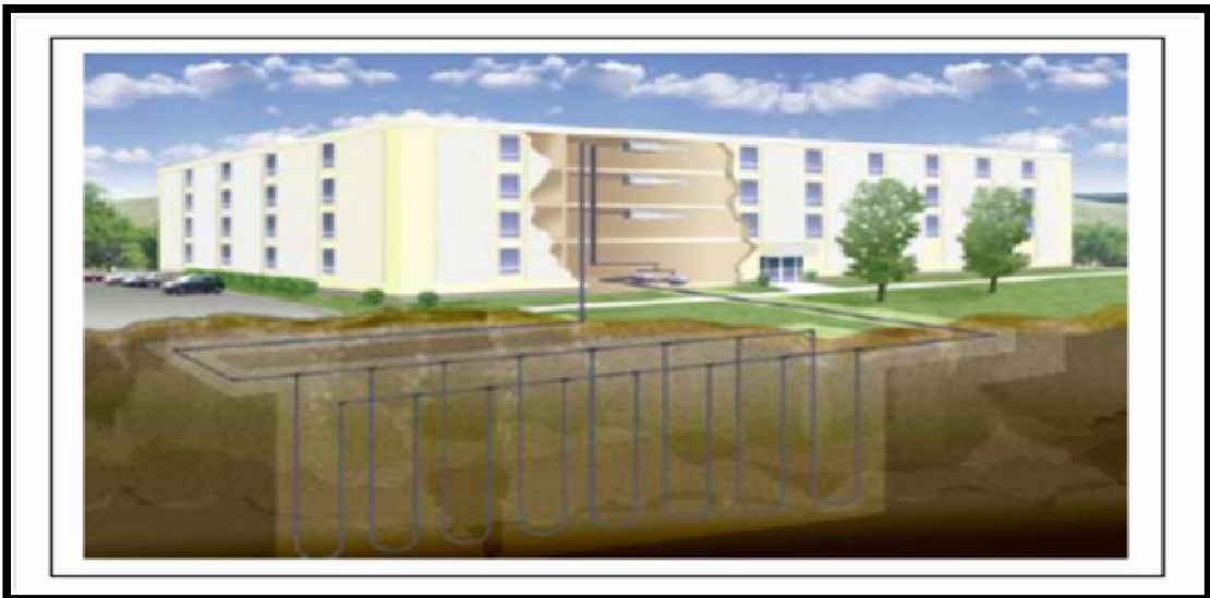
Figure (1.4) Vertical loop geothermal heat pumps [7]
