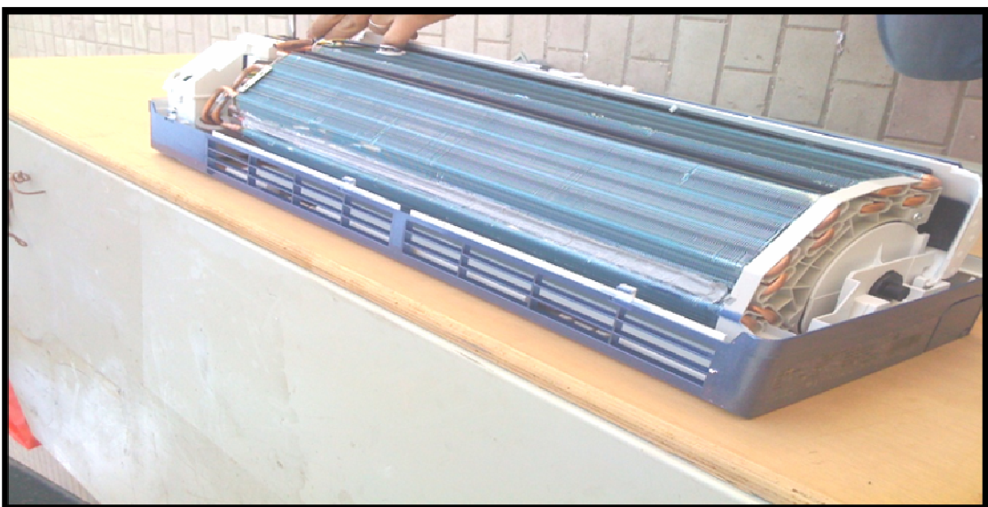
Figure (5.4) Evaporator 10000 btu/hour type (Electra)
