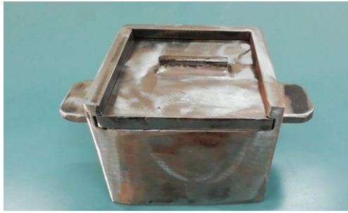
Figure 5. The manufactured carburization container.
