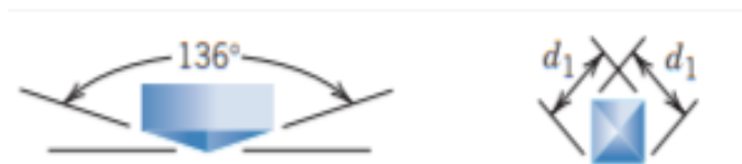
Figure 7. The side view and top view of indentation (Callister and Rethwisch, 2018).
