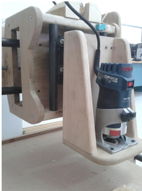
Figure 3- 2 Spindle motor installed on the Z axis of the machine.
