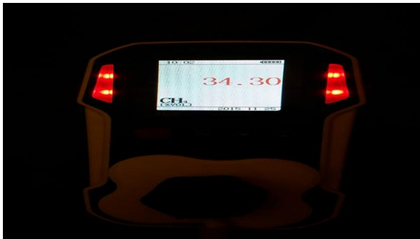
Figure 4. 13: CH 4 Measurement By Multi Gas Detector.
