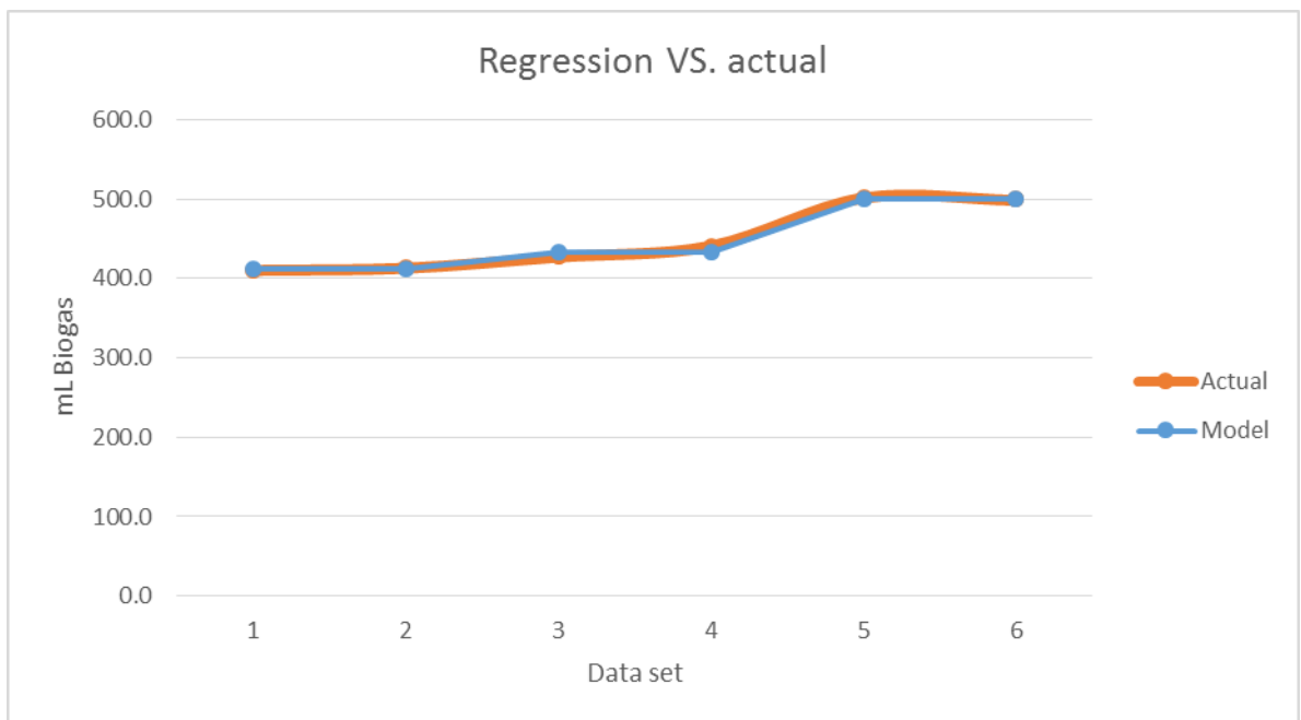
Figure 5. 20: Predicted Biogas Production (Regression Model) Versus Actual Data
