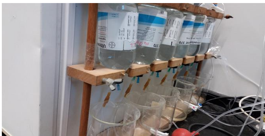
Figure 4. 12: Water Displacement Unit (Biogas Measurement).
