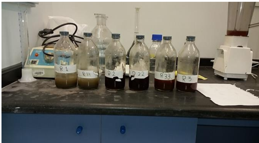
Figure 4. 11: Feed Samples in Reactors Before Inoculation.
